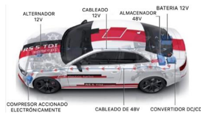
Figura 7. Audi Electric Turbo mHEV (Green Car Congress, 2014)
